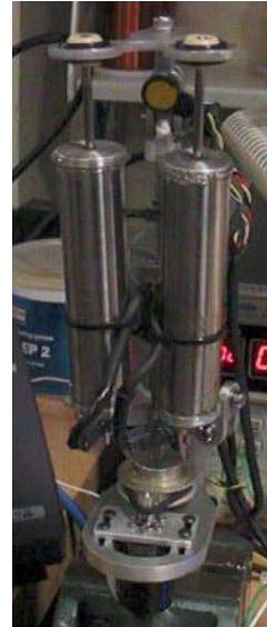
Fig. 2 The Neck Mechanism.
